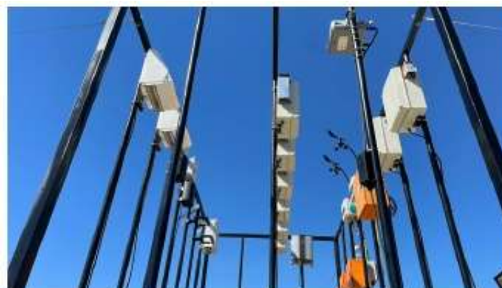
Figure 78: Example of various Low-cost air quality sensor equipment (Wernecke, et al., 2023) Growing KwaZulu-Natal Together
